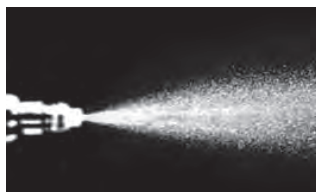
Injector spray pattern after P.i. treatment.
